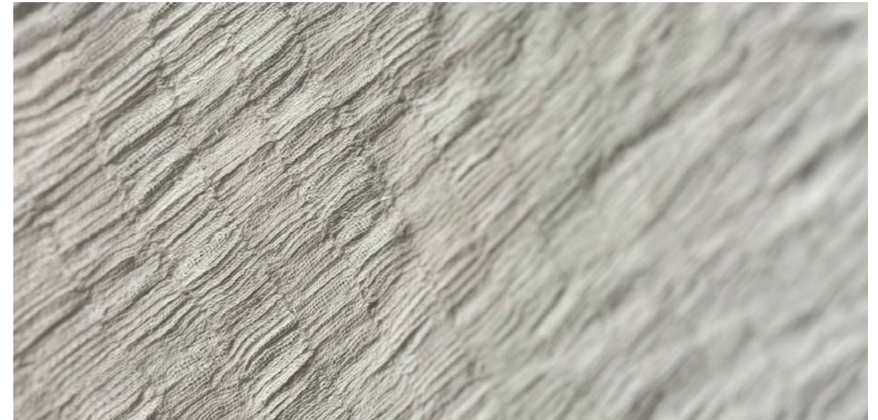
Figure 53. Double plain inlay structure - overtwisted yarns. TC2 hand-operated electronic Jacquard sampling loom
