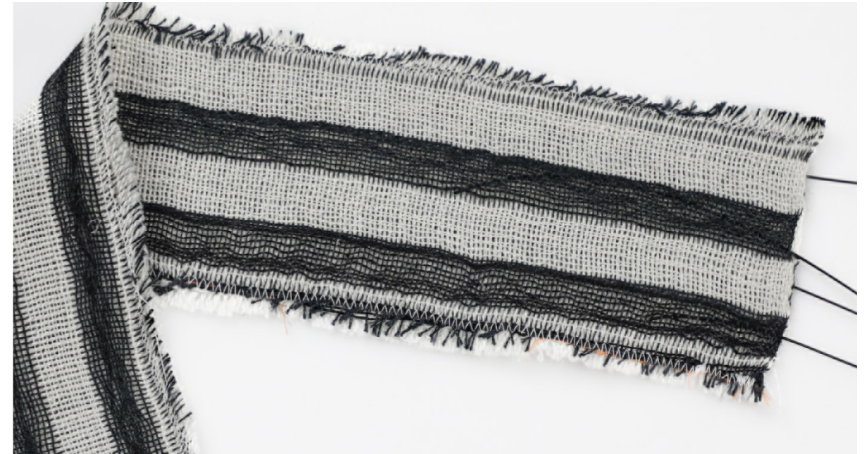
Figure 51. Double plain inlay structure. Manual shaft loom
