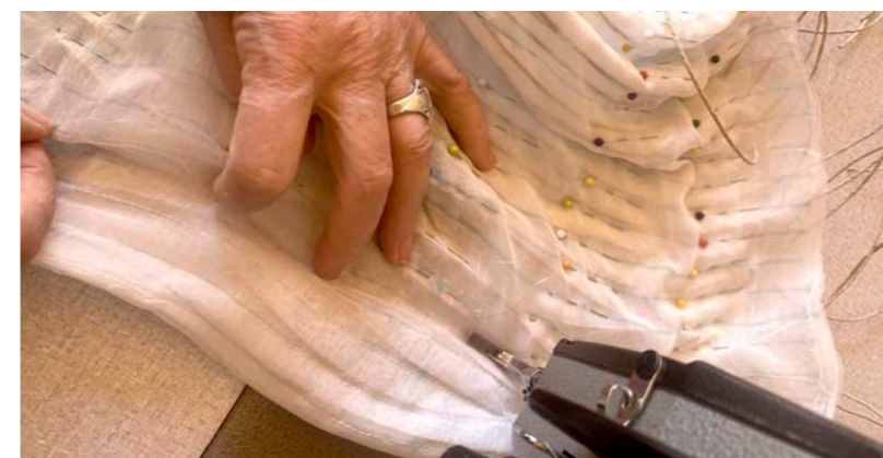
Figure 57. Manually replicating double plain inlay structure
