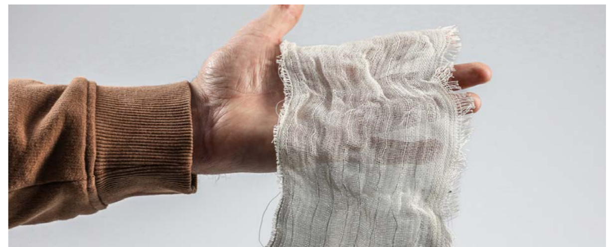
Figure 55. Density of a double plain inlay structure compared to a 4-layer plain inlay structure. TC2 hand-operated electronic Jacquard sampling loom
