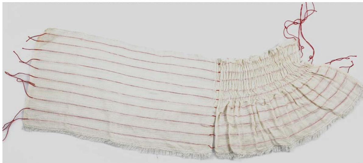
Figure 54. 4-layer plain inlay structure. TC2 hand-operated electronic Jacquard sampling loom
