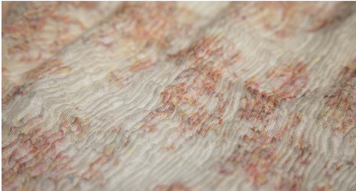
Figure 56. 4-layer plain inlay structure with overtwisted yarns. Aalto University industrial Jacquard loom
