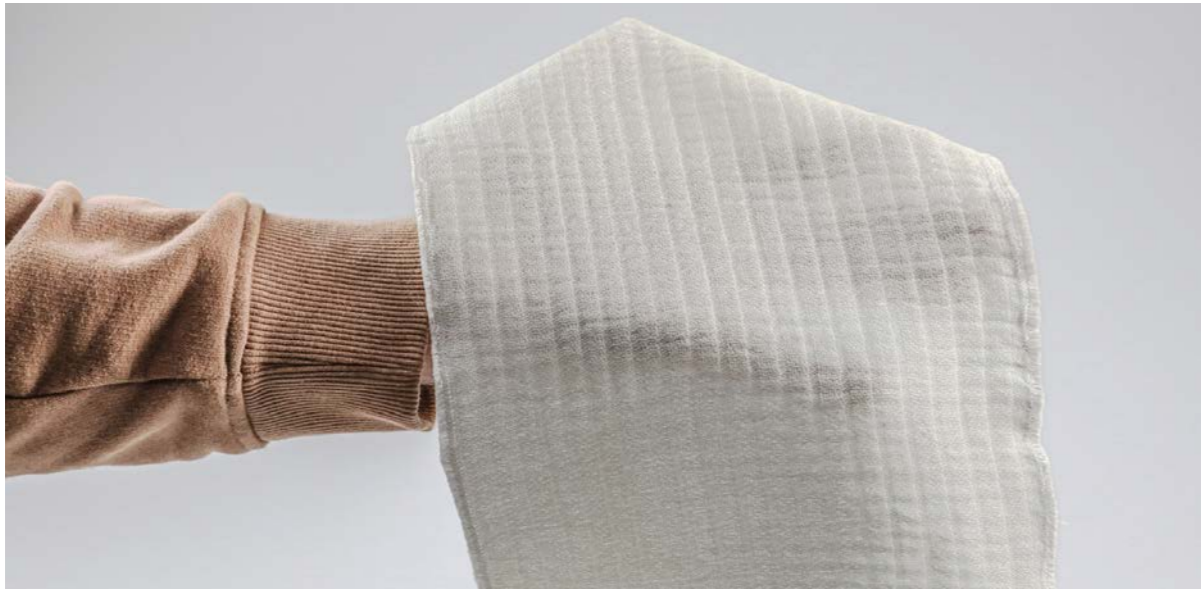
Figure 52. Double plain inlay structure. TC2 hand-operated electronic Jacquard sampling loom
