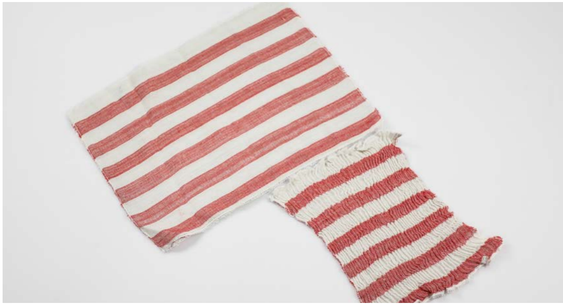
Figure 35. Overtwisted yarn effect
